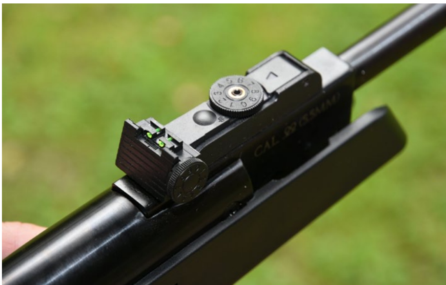
The adjustable rear sight has fibre-optic inserts.
