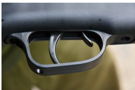
The tab in front of the trigger blade is the manual safety.
