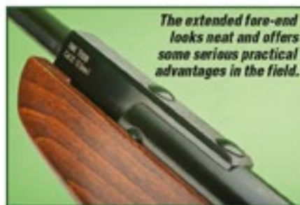
Above: The TH208's receiver is grooved for a telly and features an arrestor plate at the end.
