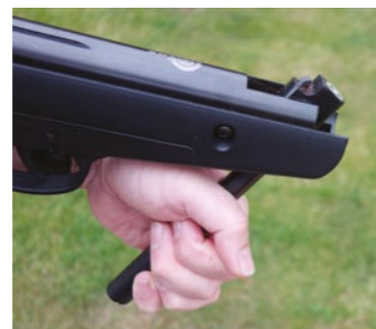
The rearsight is adjustable for windage and elevation
